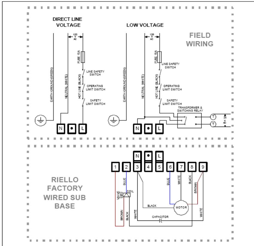
REMOTE SENSING OF SAFETY LOCKOUT: The SAFETY SWITCH in the 530SE CONTROL BOX is equipped with a contact allowing remote sensing of burner lockout. The electrical connection is made at terminal 4 (•) on the SUB-BASE. Should lockout occur the 530SE CONTROL BOX will supply a power source of 120Vac to the connection terminal. The maximum allowable current draw on this terminal (4) is 1 Amp.
