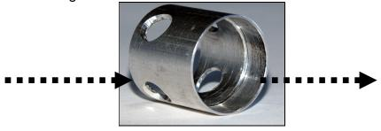
In extreme cold conditions, cover the holes on the temperature feeler gauge using foil tape. Ensure that the temperature feeler gauge is readjusted for warmer weather conditions. Failure to do so may result in burning out fan switches- not covered under warranty.
