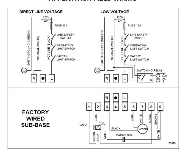
**REMOTE SENSING OF SAFETY LOCKOUT:** The SAFETY SWITCH in the 530SE CONTROL BOX is equipped with a contact allowing remote sensing of burner lockout. The electrical connection is made at terminal 4 (●) on the SUB-BASE. Should lockout occur the 530SE CONTROL BOX will supply a power source of 120Vac to the connection terminal. The maximum allowable current draw on this terminal (4) is 1 Amp.
