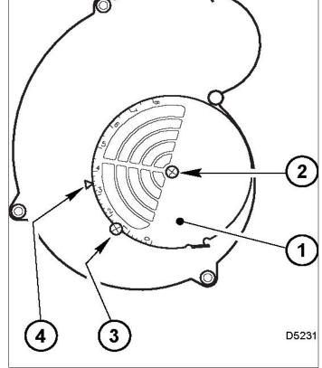
C) The final position of the air distribution adjustment plate will vary on each installation. Use instruments to establish the proper settings for maximum CO<sub>2</sub> and a smoke reading of zero.
