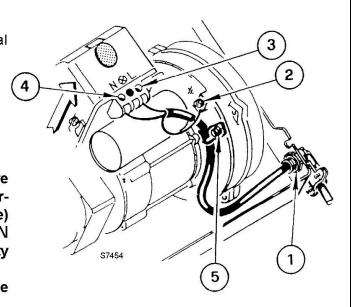
The burner may be controlled using either a DIRECT LINE VOLTAGE control circuit (120V AC 60 cycle) **OR** a LOW VOLTAGE control (24V AC 60 cycle) using a R8038A Honeywell switching relay or equivalent.
