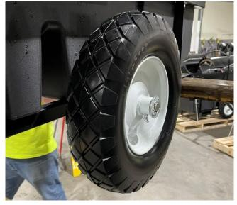
10. Slide a ¾" washer onto the axle on the far side of the axle. Slide on the far wheel (with the grease fitting facing out).
