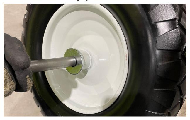
9. Slide the axle (with close wheel attached) into the unit, from the forklift side. The close wheel will now be installed on the forklift side of the unit, with the bare axle protruding from the side of the unit furthest from the forklift.
