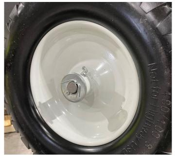
12. Gently move the wheel in and out on the axle looking for excessive play between the wheel and the frame of the unit. If there is excessive play, insert a second ¾" washer behind the wheel.
