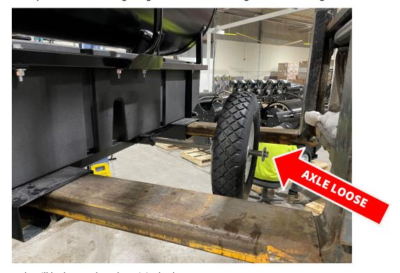
5. **NOTE**: The new axle will be longer than the original axle.
