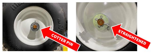
3. Remove the far wheel from the axle and save the 3/4" washer from behind the wheel.
