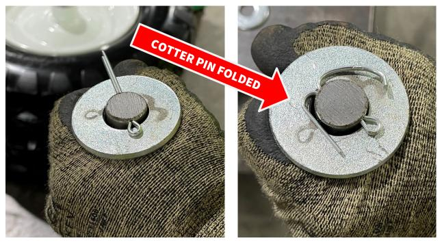
7. Slide a new wheel onto the axle shaft, all the way until it reaches the washer and cotter pin end.
