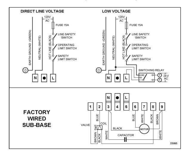
**REMOTE SENSING OF SAFETY LOCKOUT:** The SAFETY SWITCH in the 530SE CONTROL BOX is equipped with a contact allowing remote sensing of burner lockout. The electrical connection is made at terminal 4 (●) on the SUB-BASE. Should lockout occur the 530SE CONTROL BOX will supply a power source of 120Vac to the connection terminal. The maximum allowable current draw on this terminal (4) is 1 Amp.
