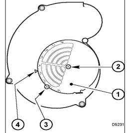
**NOTE:** Variations in flue gas, CO<sub>2</sub> and temperature readings may be experienced when the burner cover is put in place. Therefore, the burner cover **must** be in place when making the final combustion instrument readings, to ensure proper test results.
