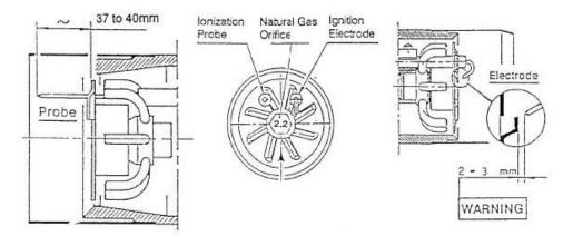
**IMPORTANT:** Do not turn the ignition electrode. Leave it as shown in the drawing. If the ignition electrode is put near the ionization probe, the amplifier of the control box may be damaged.
