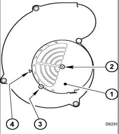
**NOTE:** Variations in flue gas,  $CO_2$  and temperature readings may be experienced when the burner cover is put in place. Therefore, the burner cover **must** be in place when making the final combustion instrument readings, to ensure proper test results.
